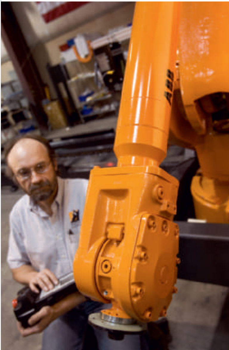
Gordon Wolschlag with the handheld controller, or teach pendant, unique to ABB.
